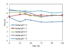
Figure.2.Final pH profile during biohydrogen production
