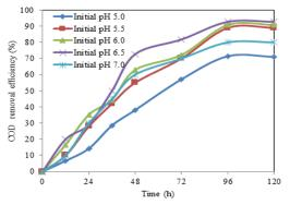
Figure.1.Effect of initial pHs on COD removal efficiency
